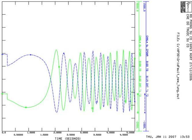
Fig. 3. Simulation of power swing in DaNang-Pleiku line, Dec 27<sup>th</sup>, 2006
