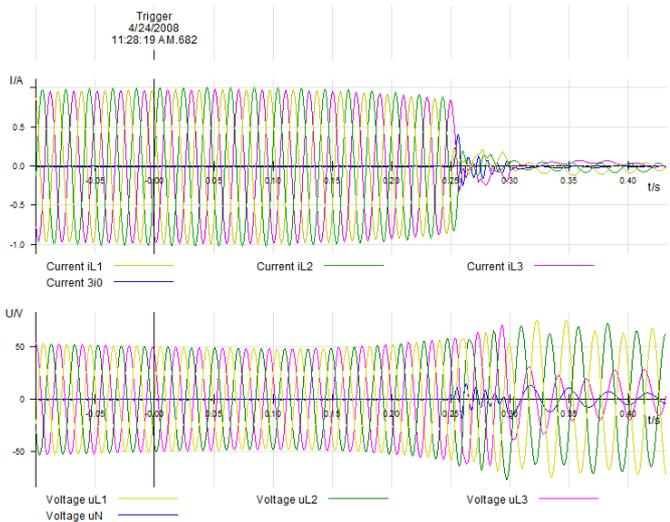
Fig. 4. Power swing recorded at Da nang 500kV Substation, Apr 24<sup>th</sup>, 2008
