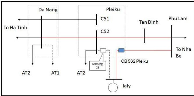
Fig. 2. Network configuration at the time of power swing, Dec 27<sup>th</sup>, 2006
